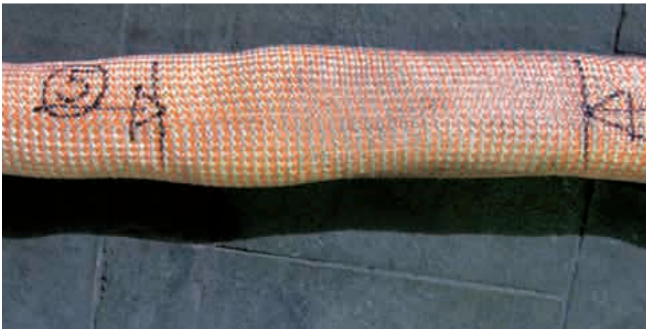
Much less damage to the protective sleeve of the Magnum-X round sling sleeve after stressing with four times the nominal carrying capacity thanks to an innovative sleeve construction
