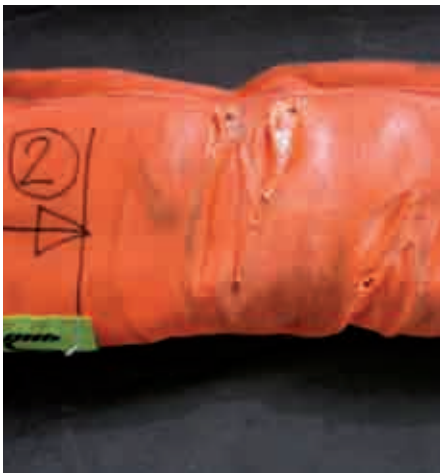
Typical impression marks after stressing with four times the nominal carrying capacity with a woven round sling sleeve
